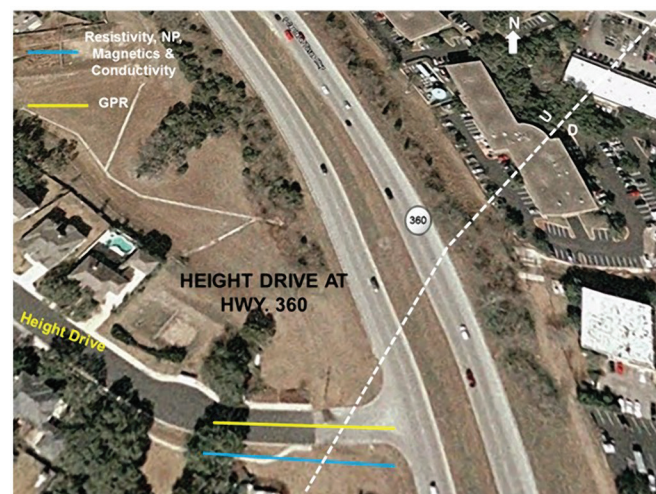
Figure 11. Site 3 map showing the locations of geophysical profile and the Mount Bonnell fault at Height Drive.
